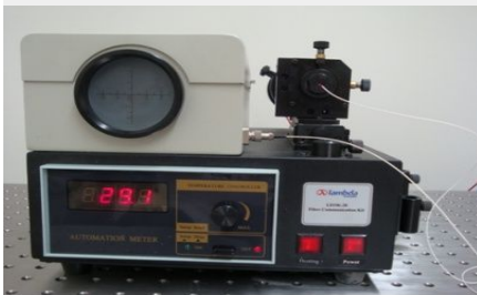
Setup for fiber temperature sensing
